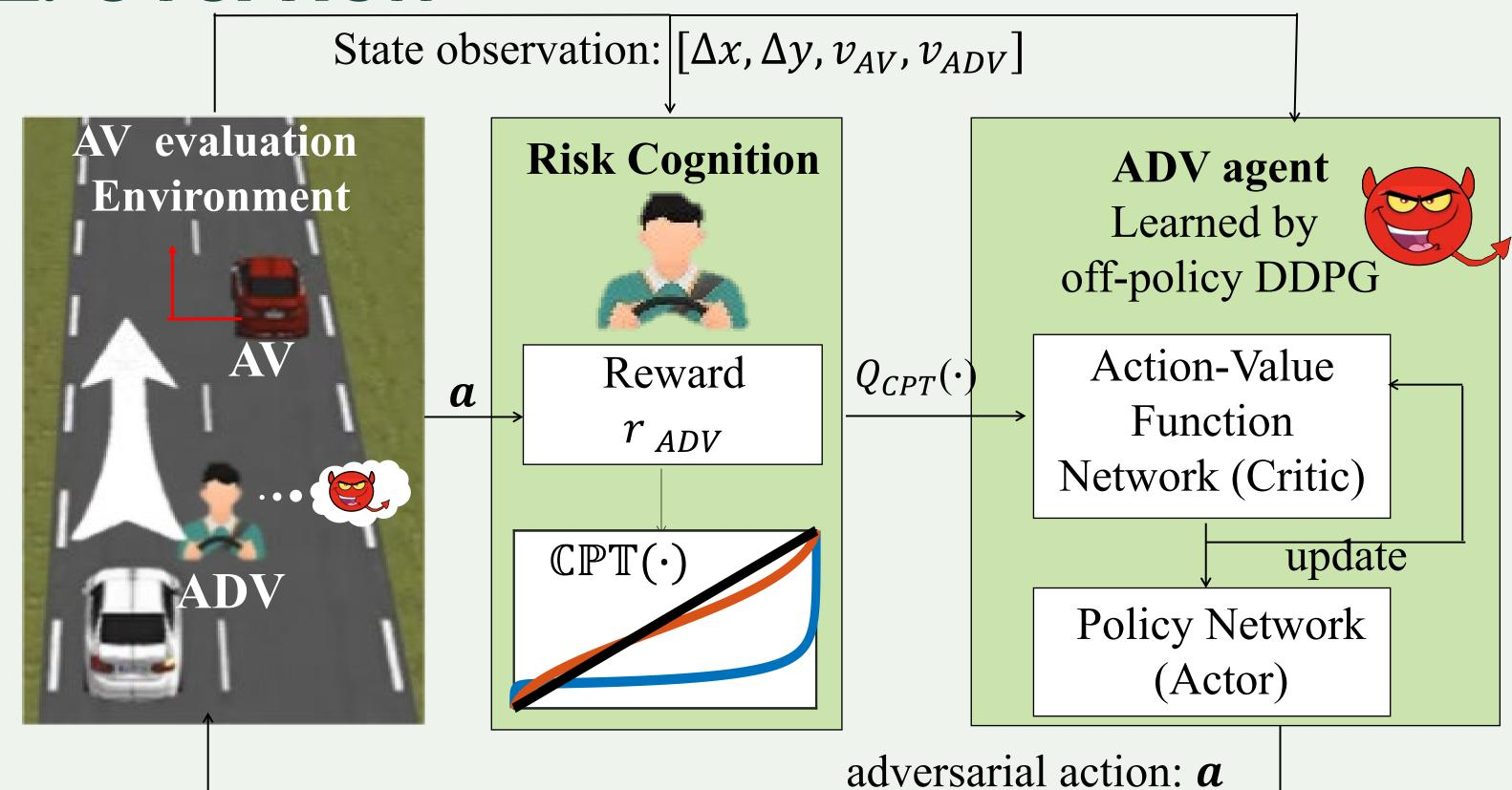
We propose a framework based on CPT to generate adversarial behavior for testing autonomous vehicle.
